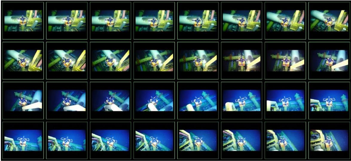
The strategy allowed the post-calibration of the ROV cameras, and accurate recalculation of the positions and attitudes of the receptacles, with final errors relative to the structure better than 0.5 mm for position and 0.1° for angles.
