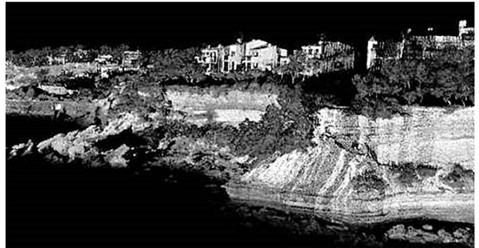
Fig. 6. 3-dimensional point cloud of the Carry-le Rouet cliffs (point cloud rendered in grey-scale using reflectance intensity)
