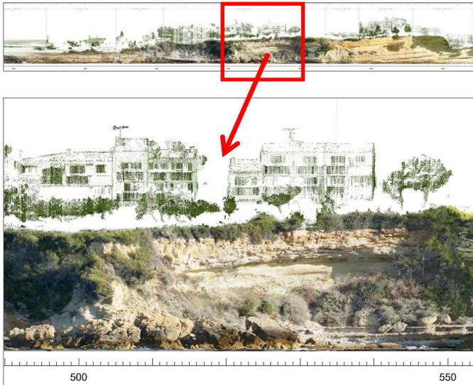
Fig. 12. Orthomosaic imagery of the entire unrolled coastline visible in one panoramic view.
