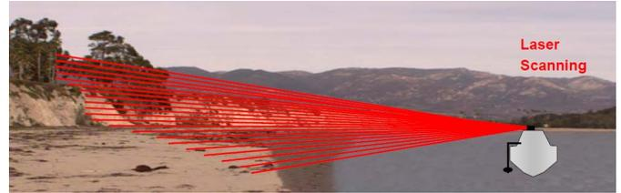
Fig. 3. Schematic of mobile laser scanning from a vessel.
