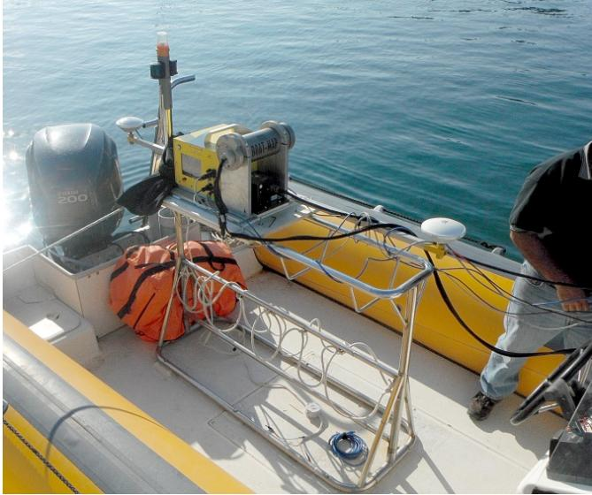
Fig. 5. Mobile laser scanning system (laser scanner, GNSS, IMU, and camera) installed in small vessel for survey.
